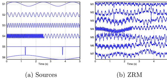
Figure 1: Simulated Signals. The ZRM montage is contaminated with Gaussian white noise, SNR=10dB
