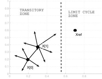
Fig. 4. From the transitory to the steady state (limit cycle). When  $L(x,t) < \epsilon$ , the system is in steady state. Otherwise, the system is in transitory state.
