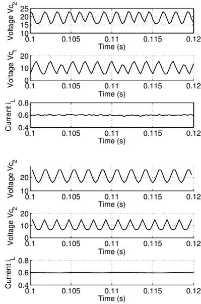
Fig. 7. Steady state voltage and current. The upper figure shows the experimental result and the lower figure the simulation result
