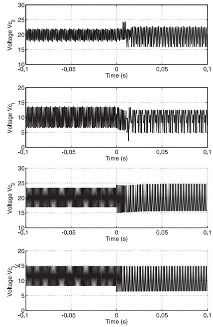
Fig. 9. Voltage response to a step in the load resistance from  $R = 20\Omega$  to  $R = 40\Omega$ . The upper figure shows the experimental result and the lower figure the simulation result.
