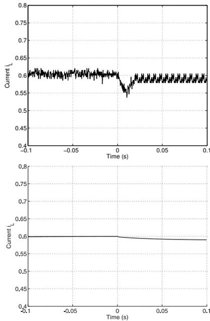
Fig. 10. Current response to a step in the load resistance from  $R = 20\Omega$  to  $R = 40\Omega$ . The upper figure shows the experimental result and the lower figure the simulation result.
