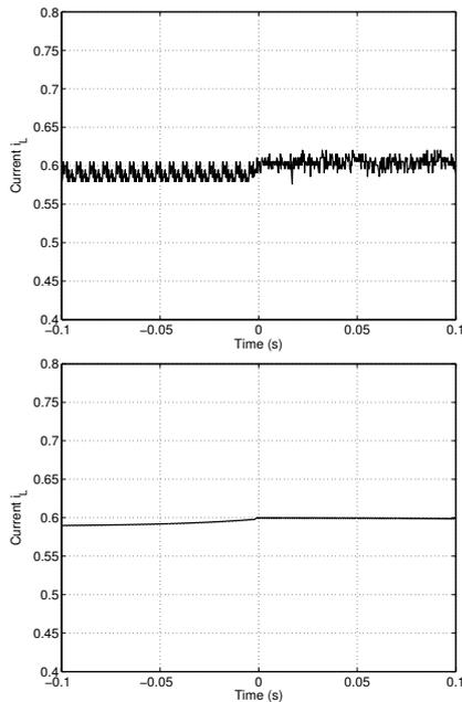
Fig. 11. Current response to a step in the load resistance from  $R = 40\Omega$  to  $R = 20\Omega$ . The upper figure shows the experimental result and the lower figure the simulation result.
