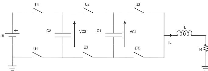
Fig. 1. Four level three cell DC/DC converter connected to an R-L load.  $u_k = 1$ , means that the  $k$ -th upper switch is closed and the lower switch is open ( $\bar{u}_k = 0$ ),  $k \in \{1, 2, 3\}$ .  $u_k = 0$ , means that the  $k$ -th upper switch is open and the lower switch is closed ( $\bar{u}_k = 1$ )
