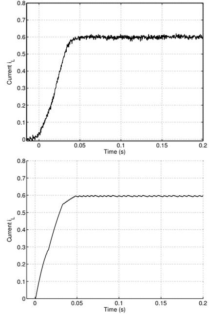
Fig. 6. Start-up transient current. The upper figure shows the experimental result and the lower figure the simulation result
