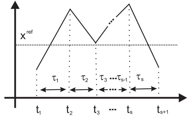
Fig. 2. Limit cycle produced by a particular sequence  $(T, I)^s$  around a given reference  $x^{ref}$
