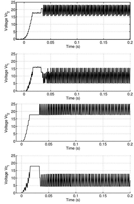
Fig. 5. Start-up transient voltage. The upper figure shows the experimental result and the lower figure the simulation result
