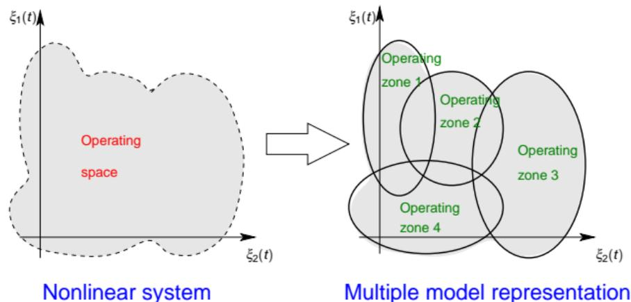
Multiple model = an association of a set of submodels blended by an interpolation mechanism
