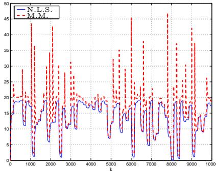
Fig. 2. Non-linear system output and linearised multiple-model output
