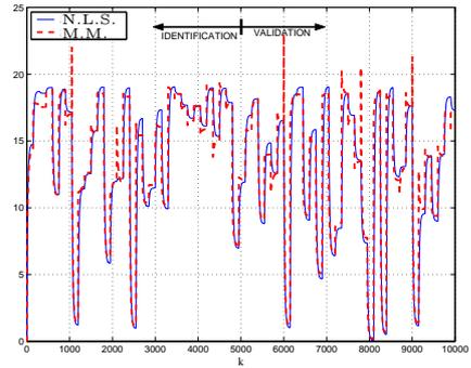
Fig. 3. Non-linear system output and identified multiple-model output
