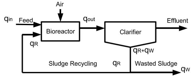
Fig. 1. The diagram of activated sludge wastewater treatment
