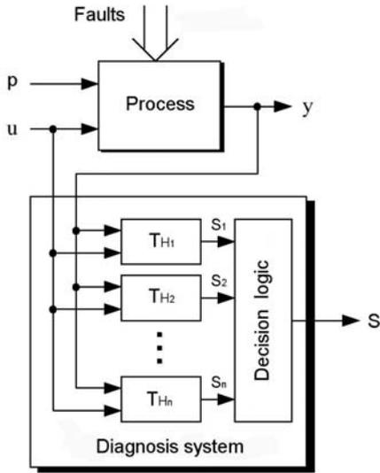
Figure 1 : Structured hypothesis tests based diagnosis system
