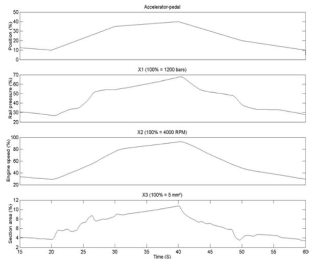
Figure 3 : Fault-free pressure control process simulation
