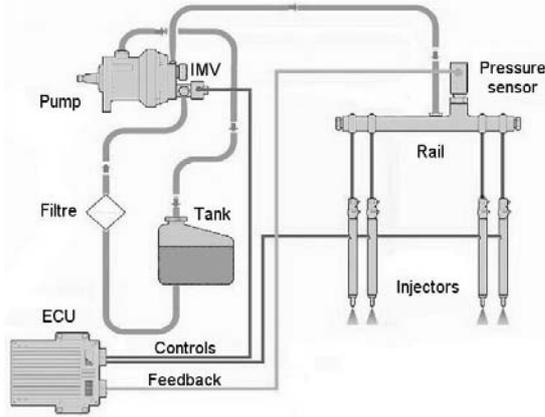
Figure 2 : Common rail diesel injection system
