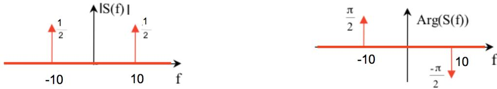
Figure 1.2: Amplitude and phase spectrum of a signal
