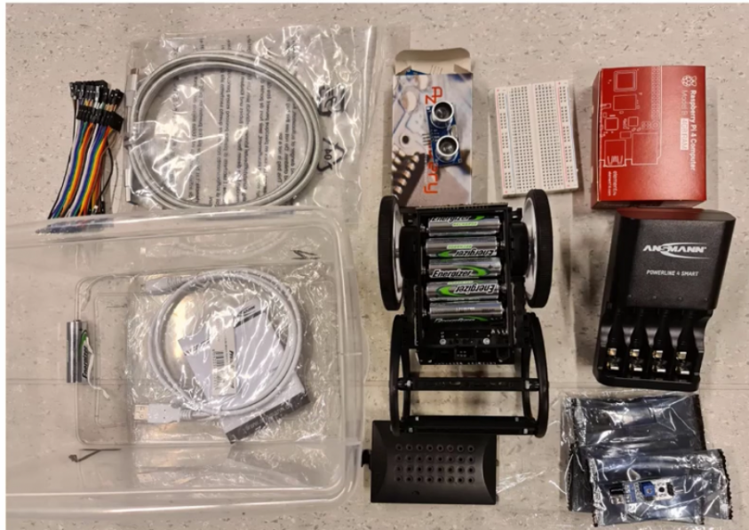
Figure 1.1: Balboa 32U4 robot from Pololu and its main components
