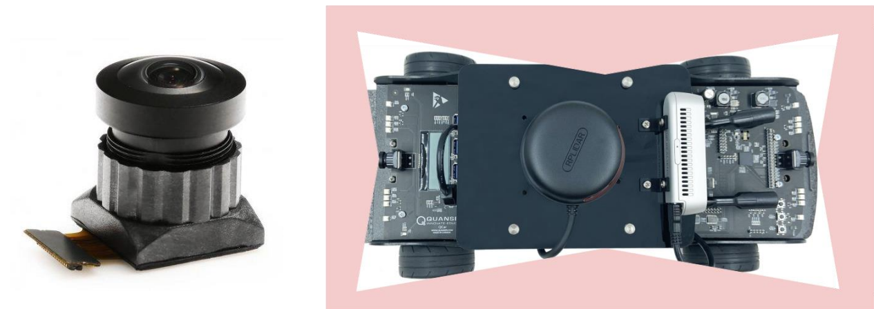
b. 360 camera coverage portraying the blind spots in white
