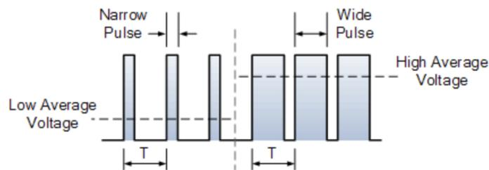
Figure 3: Illustration of Pulse Width Modulation (PWM) signals for motor speed command
