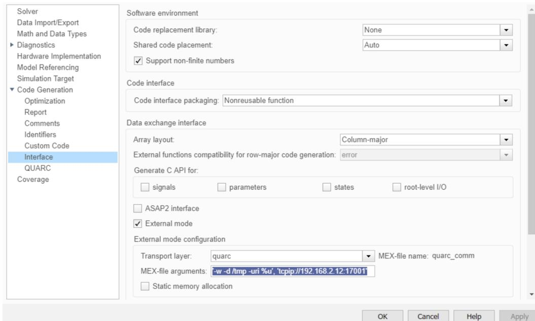
Figure 2: Qcar IP address setting for code generation.
