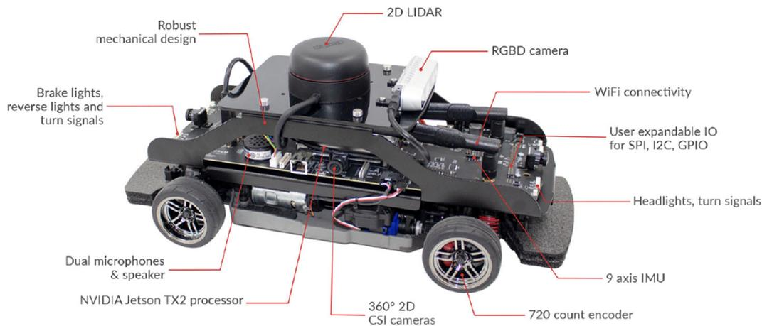
Figure 1: The Qcar and its main components.
