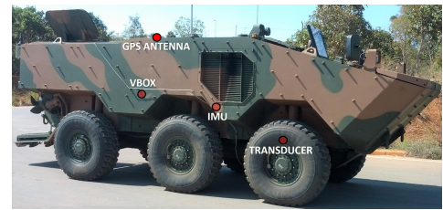
Fig. 1. Vehicle used for experimental measurements
