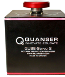
Figure 4.1: Qube-Servo 2 platform equipped with the inertia disk
