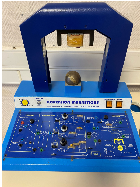
Implementation of the analogue PID controller Via electronic amplifiers
