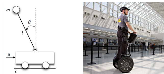
Figure 8: Simplified diagram of an inverted pendulum on a cart (left) - Segway people mover (right)
