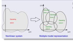
Multiple model = interpolation of a set of linear submodels
