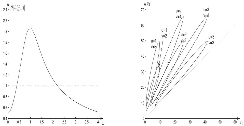
Figure 3.6: The crossing set for the system (3.31) can be identified to the left and some crossing curves of this system are plotted to the right
