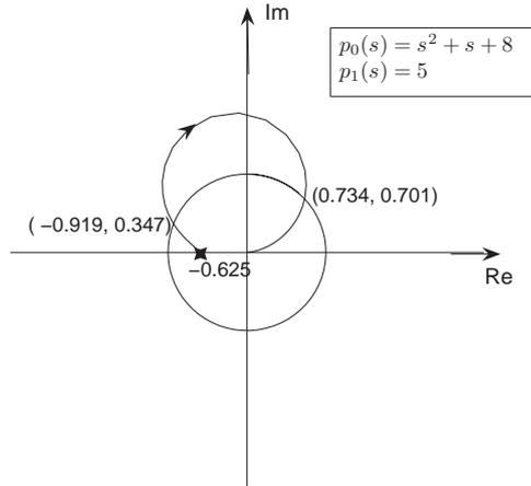
Figure 3.2: The crossing set contains two points, first crossing corresponds to a switch to instability and the second to a reversal one.
