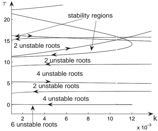
Figure 4.20: Stability crossing curves for the system given by (4.69)
