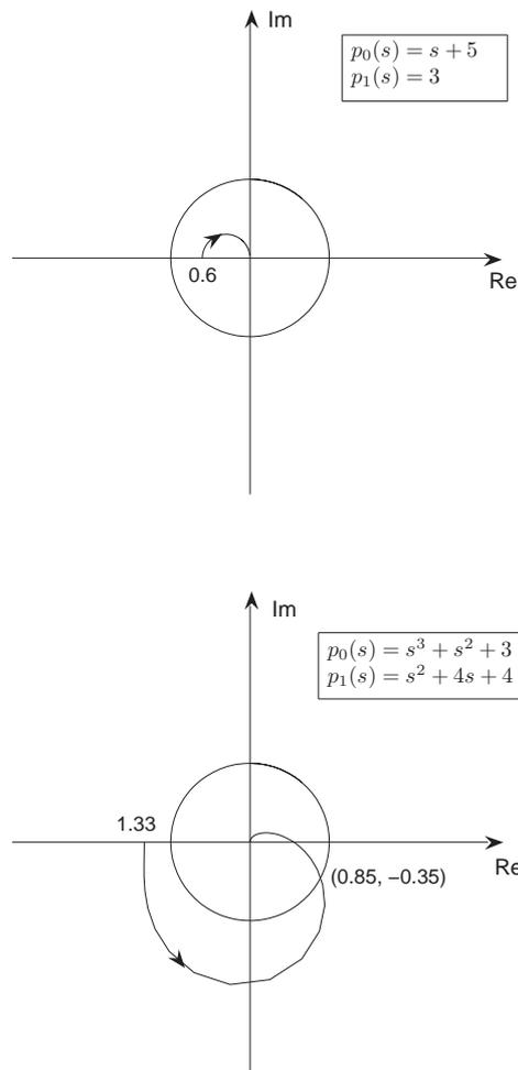
Figure 3.1: Up: No crossing occurs; Down: The crossing set contains one point and the corresponding crossing direction is towards instability.
