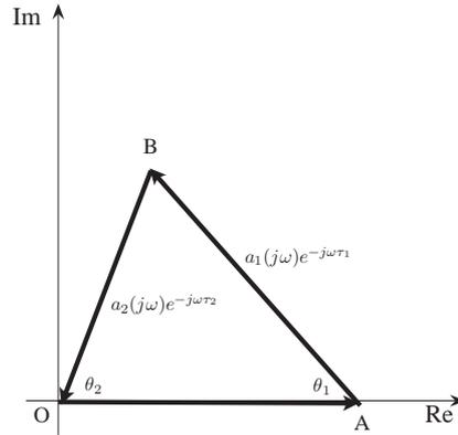
Figure 3.4: Triangle formed by 1,  $a_1(j\omega)e^{-j\omega\tau_1}$  and  $a_2(j\omega)e^{-j\omega\tau_2}$
