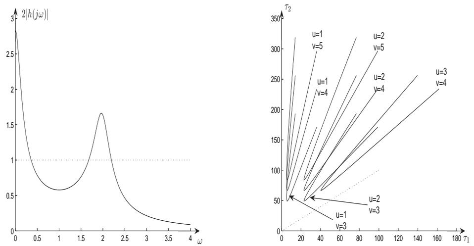
Figure 3.7: The crossing set for the system (3.32) can be identified to the left and some crossing curves of this system are plotted to the right
