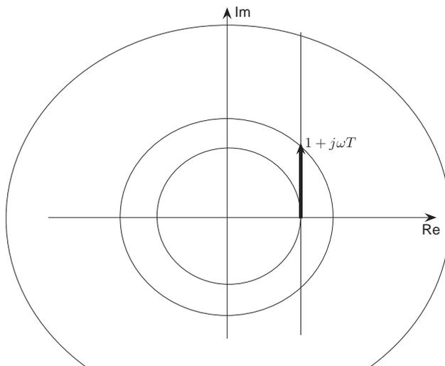
Figure 4.1: The intersection is possible only if the radius  $\left|\frac{Q(j\omega)}{P(j\omega)}\right|^{1/n}$  is larger than 1. The extreme cases for intersection are given by  $\left|\frac{Q(j\omega)}{P(j\omega)}\right|^{1/n} = 1$  or  $\left|\frac{Q(j\omega)}{P(j\omega)}\right|^{1/n} \rightarrow \infty \Leftrightarrow P(j\omega) \rightarrow 0$
