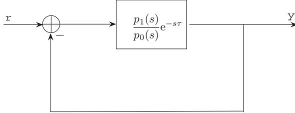
Figure 3.3: The closed-loop of  $H_0(s)$ .
