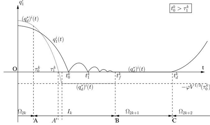
Fig. 3. The design of  $q_{1d}^*$  on the transition phases  $I_k$
