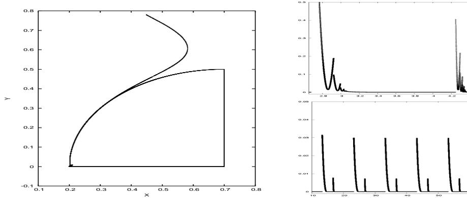
Fig. 7. Left: The trajectory of the system during 6 cycles; Right-Up: Zoom on the transition phases during the first cycle; Right-Down: The variation of the Lyapunov function on the last 5 cycles.
