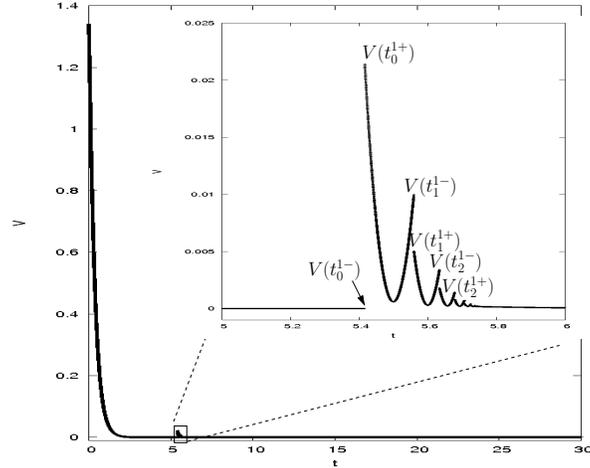
Fig. 6. Variation of the Lyapunov function for  $\gamma_1 = 8, \gamma_2 = 7$ ; Zoom: Variation of the Lyapunov function during the phase  $I_0$
