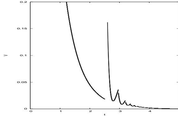
Fig. 1. Typical evolution of the Lyapunov function during one cycle of a weakly stable system.
