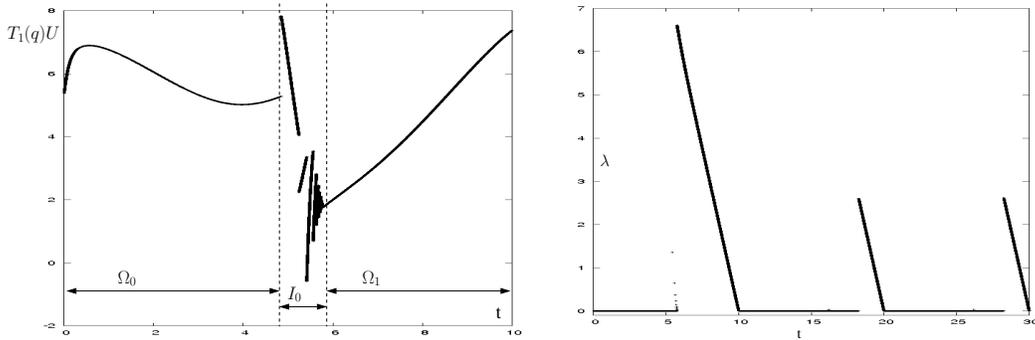
Fig. 5. Left: The switching controller on the first cycle; Right: Variation of the contact force  $\lambda$
