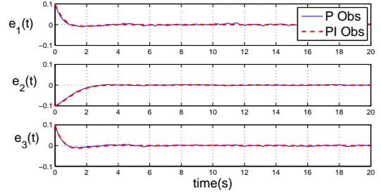
Fig. 2. State estimation errors of submodel 1
