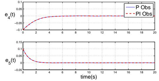
Fig. 3. State estimation errors of submodel 2
