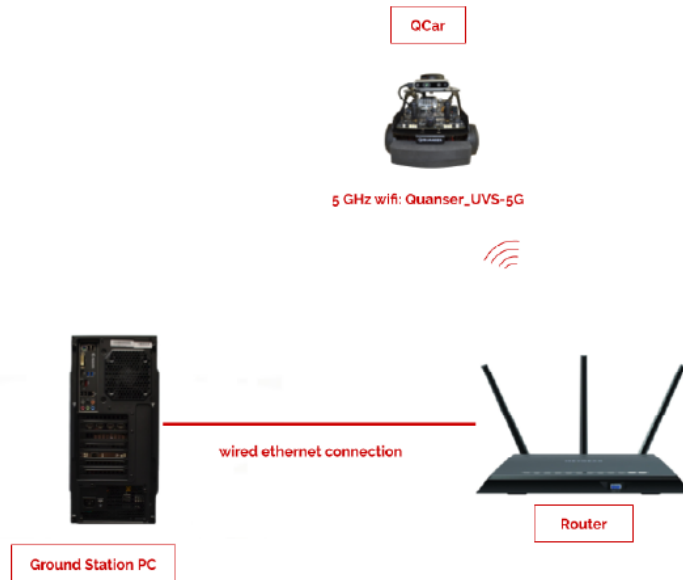
Figure 9: Communication between a computer with QUARC installed and the QCAR
