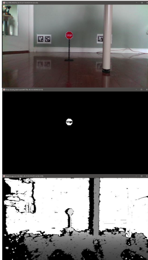
Figure 49: RGB image (top) — Thresholded image (middle) — Depth image (bottom)
