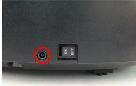
Figure 1.4: Button on/off and plug for the battery charger
