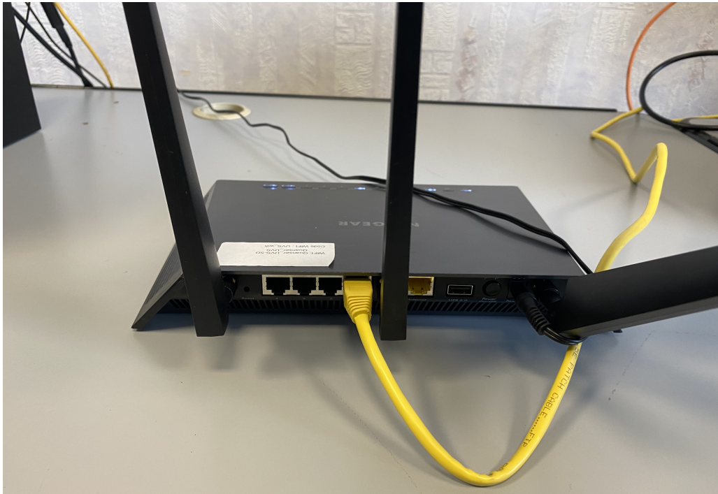
Figure 1.7: Wired connection between the router and the PC
